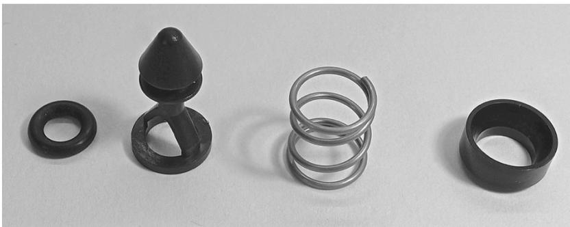
**This completes the disassembly of the EV50 Medium Pressure hose.**
